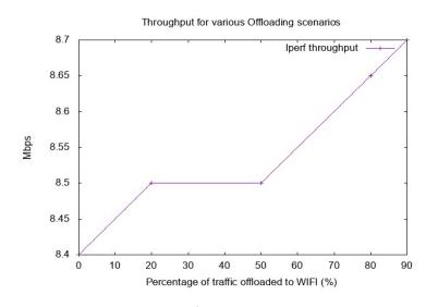
**Conclusions:** The benefits of WiFi and LTE aggregation in providing higher performance and throughput to end users has been studied. Overall, for big percentages of the offloaded traffic to WiFi, an increase of over 5% is observed.
